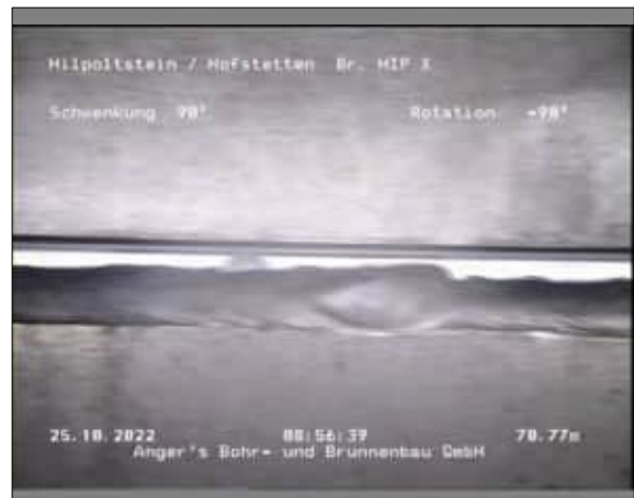
Foto: 1_1_30_A.JPG 70,77m, OK Filterrohr
